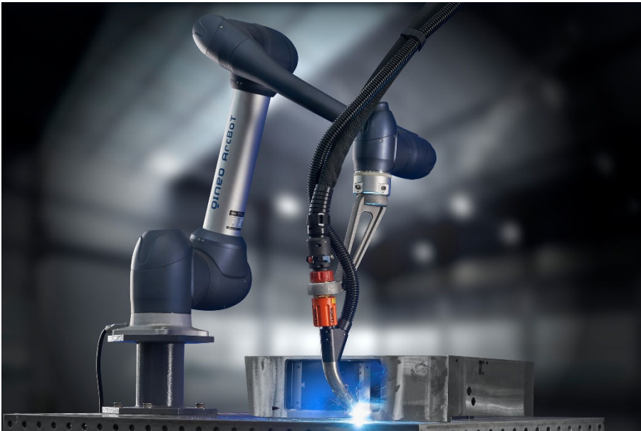
Photo 3: The QINEO ArcBoT relieves employees and ensures consistent, reproducible welding quality.
