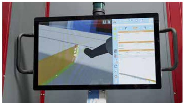
Photo 2: The system converts the stored data from the scanner into a 3D model.
