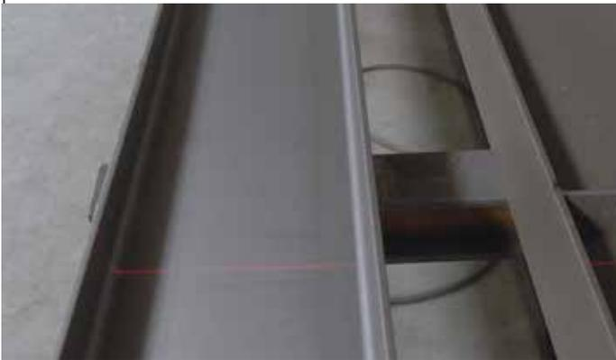
Photo 1: The laser scanner scans the work surface of the component and saves the result.
