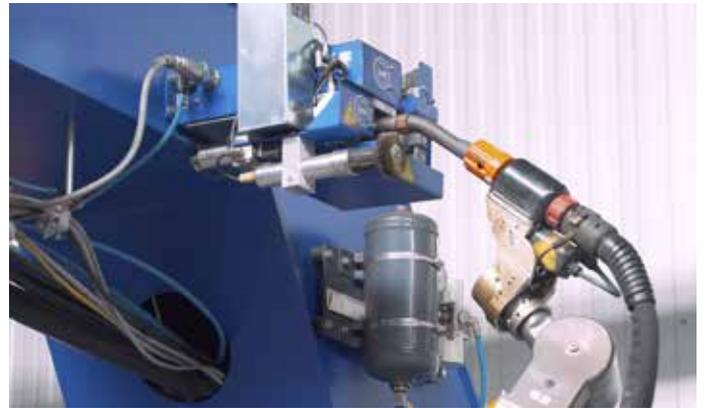
Photo 4: The robot system also includes a fully automatic welding torch cleaning system.
