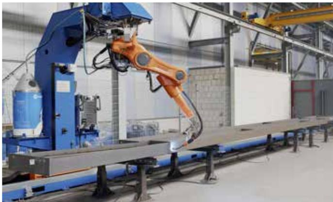
Photo 3: The robot is mounted overhead on a floor-mounted linear track.
